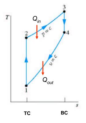
Cut-off ratio:  $r_c = \frac{v_3}{v_2}$
